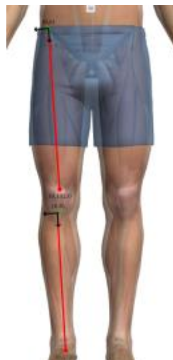
Figure 7– Example of the coordinate system on upper and lower right leg. Green dots represent origins of the surface coordinate systems. Only the vertical axis is shown. The red dots indicate the ends of the vertical axes. The circumference axis runs around the body part in a clockwise fashion. Dots are located at anatomical landmarks.
